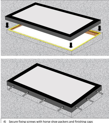
Secure fixing screws with horse shoe packers and finishing caps continuously all the way around securing the aluminium frame in place.
