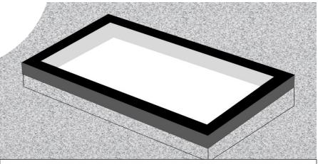
4) Internally finish by plaster boarding over the timber and straps leaving at least a 10mm gap from the top of the plasterboard to glass.
