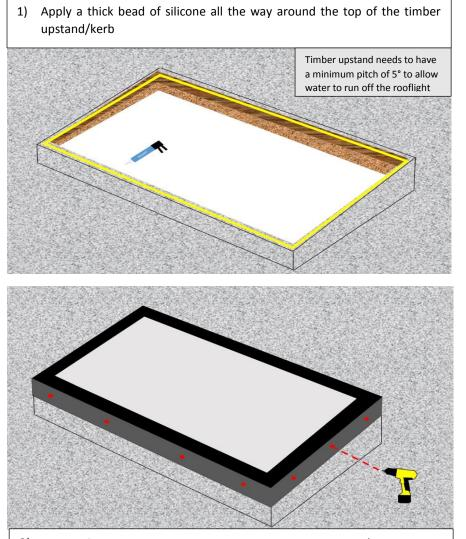
3) Pre drill fixing holes through aluminium and timber upstand/kerb at 100mm from each corner and then at regular intervals.
