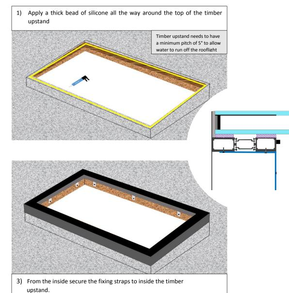
2) Position the Rooflight over the upstand ensuring that the fixing straps have been fixed to underside of frame (refer to diagram centre).
