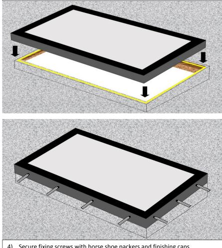
4) Secure fixing screws with horse shoe packers and finishing caps continuously all the way around securing the aluminium frame in place.
